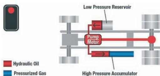
Figure 1: Storing braking energy.
