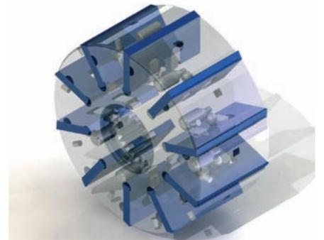
Figure 5: Transparent rotor showing vane restraint.
