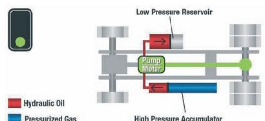
Figure 2: Releasing energy during acceleration.
