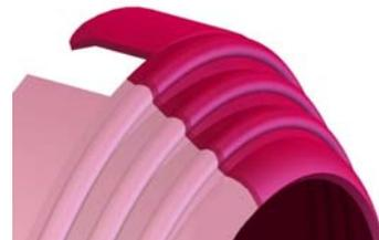
Sealing Ribs with Loctite coating
