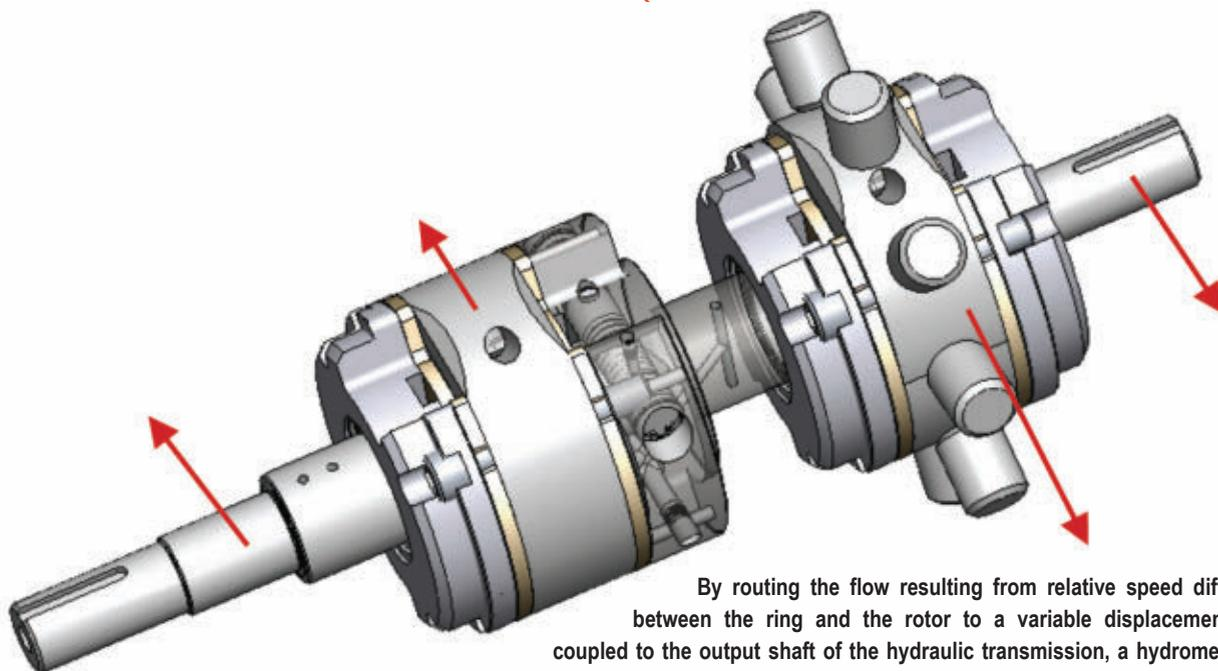
By routing the flow resulting from relative speed differences between the ring and the rotor to a variable displacement motor coupled to the output shaft of the hydraulic transmission, a hydromechanical transmission, shown here without an external housing, is formed.
