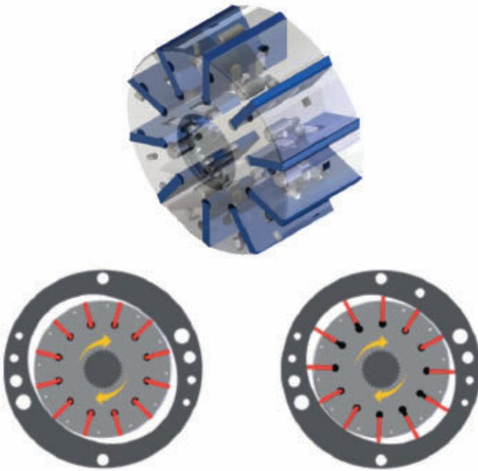
The pressure-controlled hydraulic transmission has a clutch feature. For each vane, there is a pin driving a ball. By providing pilot pressures to these pins, the vane can be fully retracted, decoupling the output shaft from the input shaft and making the transmission function as a clutch. The figure at top shows the vane structure and the bottom figures (left to right) illustrate the idle and transmission mode.
